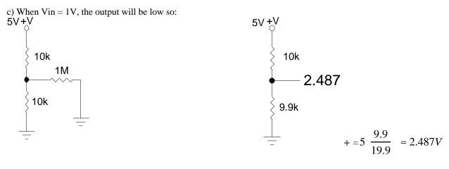
• will be 1 diode drop higher: 2.487V + 0.6V = 3.087V
