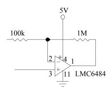
To compute the required offset, look at Vin and Vout at 100%RH: 100k
