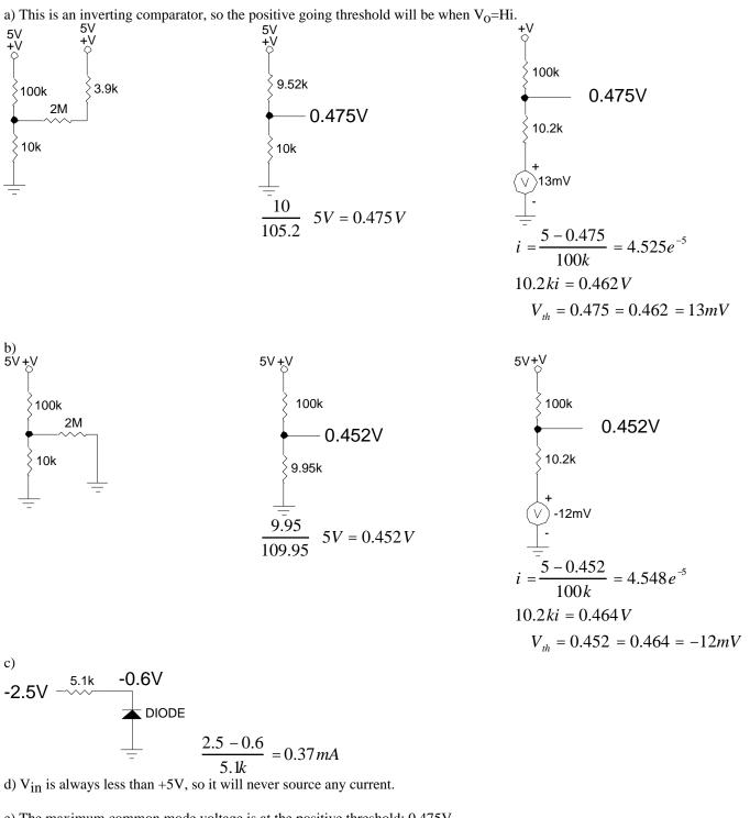
e) The maximum common mode voltage is at the positive threshold: 0.475V
