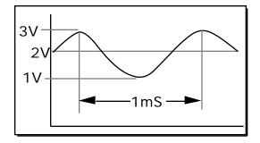
Given the input waveform shown above, design a circuit to remove the DC offset with minimal impact on the waveform.
