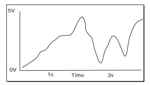
Assume the signal above is the input to a 74LS14. Overlay the output behavior. Justify your drawing.
