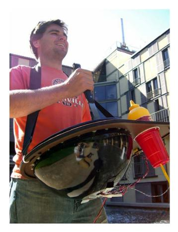
The helm is designed to simulate the classic barbeque experience. There is an actual barbeque incorporated into the helm as a well barbeque utensil and condiments. The user manipulates the barbeque utensil and condiments to maneuver the boat and to squirt water. The helm also communicates information to the captain through the use of dynamic graphical indicators which are controlled by servos. There is also a siren to indicate when the boat is "stood down".
