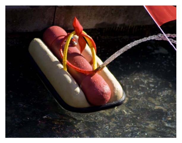
Our two-independent-propeller drive train worked in tandem with our "bun-shaped" hull allowing us to achieve this goal of combined speed and maneuverability. For water dispensing, the boat featured two bilge pumps which directed the water through two nozzles mounted to the front of our craft. The boat also featured a sealed midsection to house all of the electronics.
