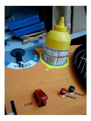
The helm also features two "special" buttons. They are simply two push buttons which can be used to control "special" features the boats may contain. For example, our boat had a siren which could be activated using these special buttons.
