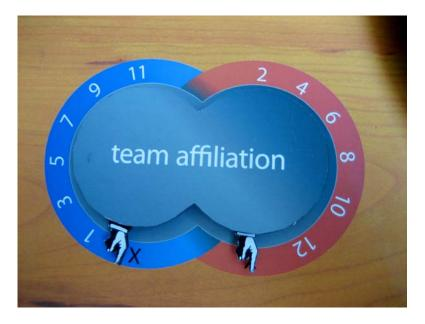
The helm uses servo controlled indicators to communicate the current active base as well as the number of the boat the helm is currently controlling. The servos are mounted underneath the main table surface and have arrows mounted to them. The servos rotate the arrows to various positions to point at the necessary graphic to convey the appropriate information.
