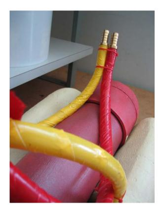
The boat features two 500 gallon per hour bilge pumps that provide some serious water dispensing capabilities. The pumped water runs up to the top of our boat through vinyl tubing and is then forced through a brass nozzle. The nozzle was sized such that it gives us a fairly long range (~12 feet) without compromising our sizable volumetric flow.
