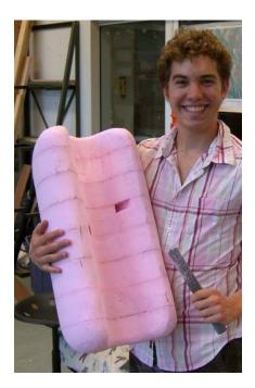
The hull is constructed of closed-cell foam which was carved into its delicious bun shape. The underside of the hull is shaped so that there are two pontoons on either side to help stabilize the boat. The hull also features cutouts on the underside to house the drive train components as wells as the bilge pumps for water dispensing.
