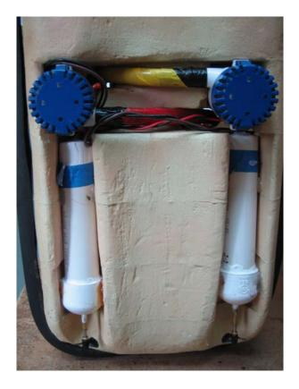
Our drive consists of two independent dc motors each driving their own propellers. The motors are housed inside sealed PVC pipe and have drive shafts exiting through grease-sealed bushings. These drive shafts are connected to RC boat propellers. The use of the two independent motors allows the boat to go backwards, forwards and rotate in place.
